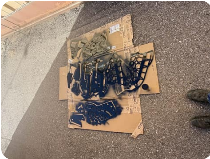
Painting CNC'd structural parts
