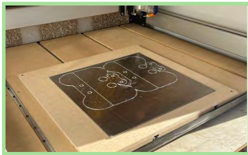
CHASSIS BEING MILLED
